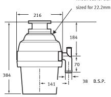
Knock-out for dishwasher drain connector sized for 22.2mm I.D. rubber hose
