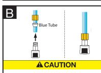
**Property Damage:**Do not over tighten brass nut.
