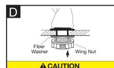
**Property Damage:** Do not over tighten the plastic wing nut.
