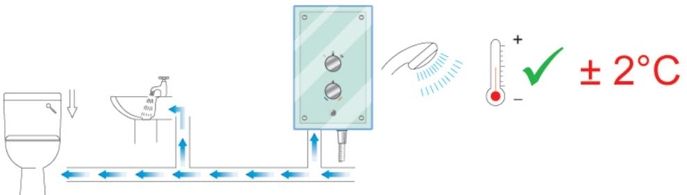
Water inlet pressure fluctuations due to other draw offs (e.g. flushing toilet). Shower temperature will be controlled to within  $\pm 2^{\circ}\text{C}$  of the set temperature provided that the supply conditions remain within the required operating parameters (refer to section: '**Specifications**').
