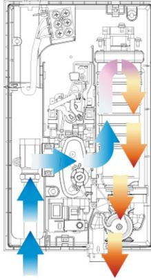
Heated water is produced by adjusting the flow of cold water passed through a heater tank.
