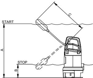
Fig. 7 Min. Float Switch Movement
