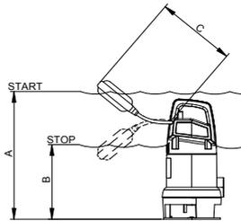
Fig. 8 Max. Float Switch Movement
