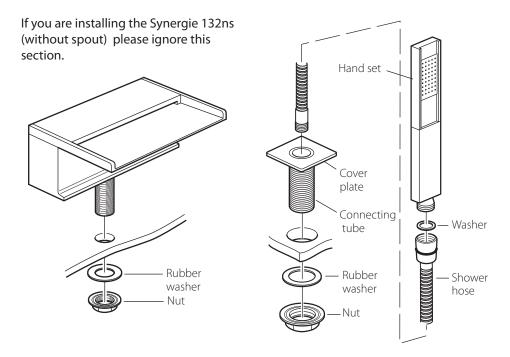
Position the spout in place , and from the underside slide on the rubber washer and nut. Tighten the nut to clamp on the spout.
