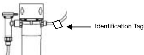
22. Next take the middle hose out of the tap base (not identified with tag) and push into the brass check valve elbow until the stop is achieved.
