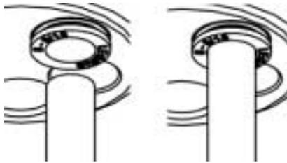
8. The product comes with ease of installation push fit connectors! Take both of loosely supplied hoses and simply push into the tap body. Push into base of the tap body until stop is achieved.
