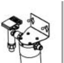
17. Once assembled offer under the sink (usually in a kitchen cupboards) the cartridge to find its best location, ensuring allowance is made for the pre assembled electronic box. Likewise be aware that to replace the cartridge you have to unscrew, so sufficient room below the cartridge is required to remove the cartridge. Note the cartridge can be located in a vertical or horizontal manner.
