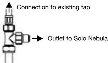
15. The cartridge head has already been semi-assembled with brass check valve elbow in place on the inlet of the cartridge head and a plastic connection piece on the outlet of the cartridge head. These have both been assembled to a defined torque and therefore should not be removed by anyone other than a BRITA or PEGLER approved installation engineer.
