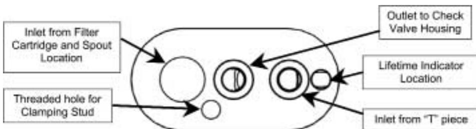
**IMPORTANT NOTE:** In any event of installing a plastic hose into the incorrect push-fit connection - to remove press the black release collar around the push-fit and pull out hose.
