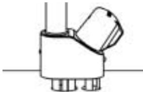
10. Once loosely in-place, check again that handle and spout movement is not obstructed.
