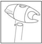
6. With the showerhead height adjuster lever set a 3 o'clock and the showerhead holder in the upright position, slide the assembly onto the rail. Tighten to the rail by turning the lever.
