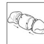
**5.** The three components that comprise the Handset Height Adjuster assembly are produced with alphabetical 'A's and 'B's moulded into the end section of each part. Simply just match the
