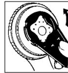
1. Engage the key into the spray cartridge recesses and turn anti-clockwise to unscrew.
