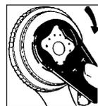
7. Refit cartridge to the showerhead and tighten with the spray key.
