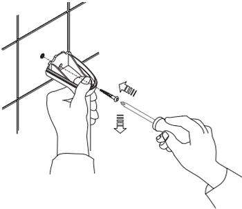
First fix bottom Slide Bar Support and fully tighten the screw\*. Then fix the top Slide Bar Support whilst pressing it down, to keep the whole assembly together.
