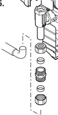
For back inlet use soldered elbow.
