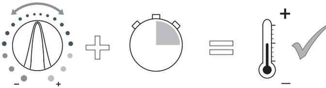
Allow 10-15 seconds for any temperature adjustments to reach the handset.
