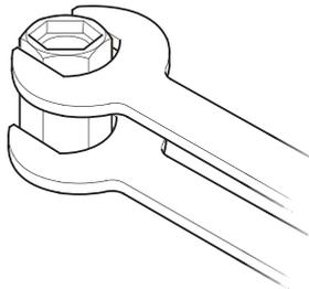
Hold a wrench across the flats of the plastic connector. Unscrew the Filter using another wrench as shown. Clean or renew the Filter as necessary. Refit in reverse order, making sure the Filter is screwed fully home.
