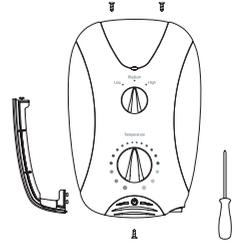
Remove three screws, Cover and Service Tunnel. Small rubber ball should be loose in the Case.
