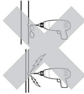
**CAUTION! Do not** drill into buried cables or pipes.
