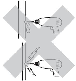
**CAUTION!** Do not drill into buried cables or pipes.
