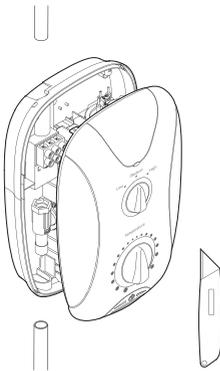
Remove Cover and determine supply pipe position.
