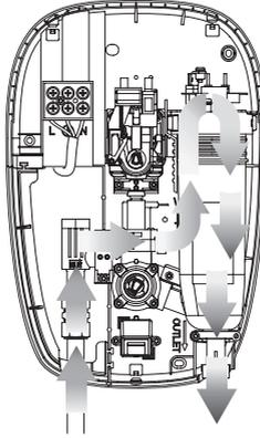
Hot water is produced by passing cold water through a heating tank.
