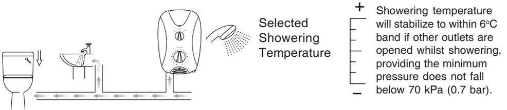
Water inlet pressure fluctuations due to other draw offs (e.g. flushing toilet) will cause the showering temperature to increase.
