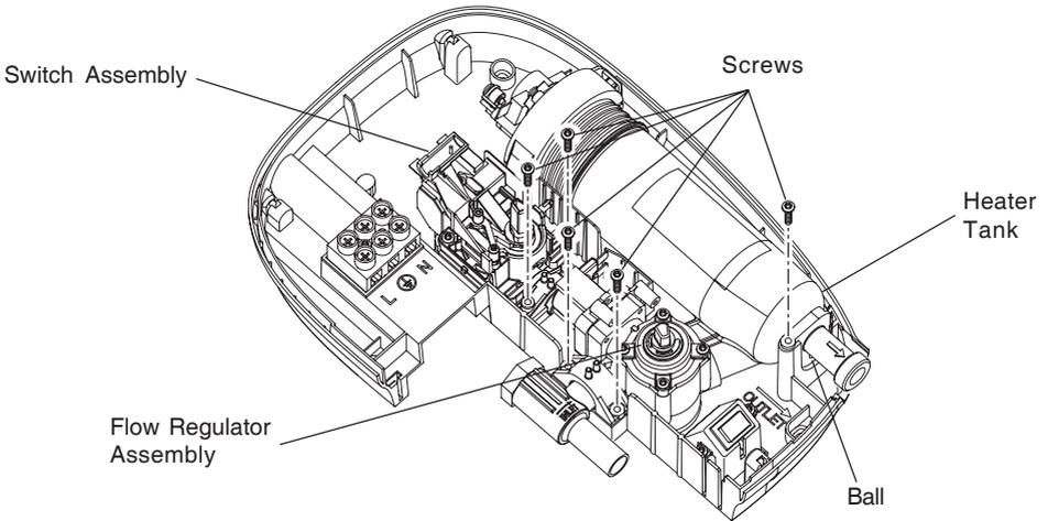
Remove the five screws and lift out the Switch, Heater Tank and Flow Regulator assemblies.
