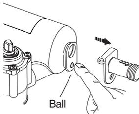
Using your finger, push the ball back into the hole in the Heater Tank assembly. **DO NOT** remove the 'O' seal.
