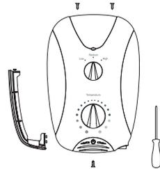
Remove three screws, Cover and Service Tunnel.
