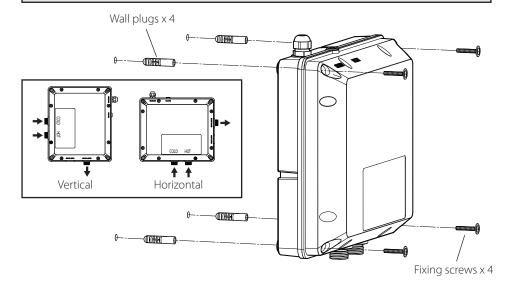
**Warning!** Please check for any hidden cables and pipes before drilling holes in the wall. The Control box can be installed either vertically or horizontally (see above).
