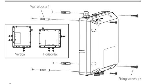
Warning! Please check for any hidden cables and pipes before drilling holes in the wall. The Control box can be installed either vertically or horizontally to a wall (see above) or flat if installed above the ceiling.
