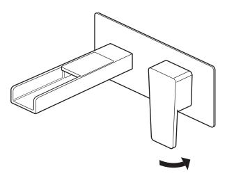
Turning the handle anti-clockwise will actuate the flow of water and progressively increase the water temperature.
