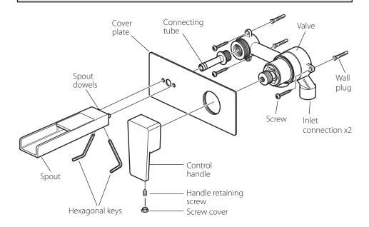
Before installing your new mixer, flush through the pipework to ensure removal of debris, turn off the water supply.
